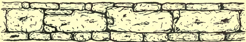
FIG. 3.—DETAIL OF MASONRY, ORAN ROUND TOWER.
